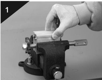
The GolfWorks Value Shaft Extractor was designed to fit in most standard vises. Simply place the shaft saver clamp into a standard vise as shown. Be sure the edge of the shaft saver clamp is even with the edge of the vise.
