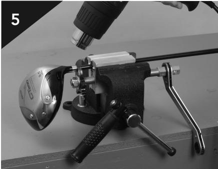
Apply heat to the hosel area using a heat gun. It is recommended to use a heat gun when removing graphite shafts. The heat gun will heat the area slower, but will be much less likely to damage the finish of the club or damage the graphite shaft.
