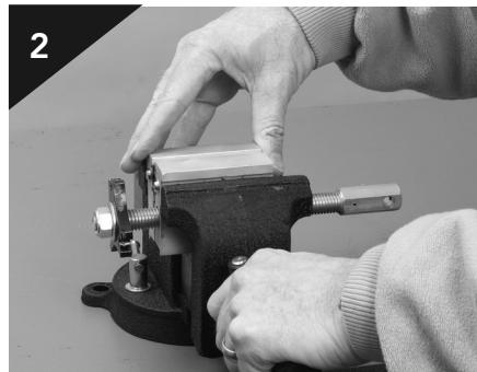
Tighten the jaws of the vise securely around the shaft saver clamp.
