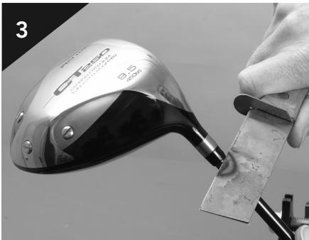
Before you place the club into the shaft saver clamp, be sure to remove the ferrule. Once the ferrule is removed, you can place a small 3/4" piece of masking tape around the shaft at the top of the hosel (the same area the ferrule occupied). This step is optional,
